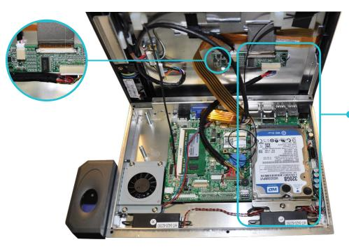
Cable Free Area, make sure LVDS and MSR cable are not caught up between the HDD and the front bezel assembly.
