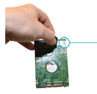
Pull one side of the plastic cover and remove the screw, pull the other side of the plastic cover and remove the second screw.
